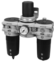
Filter + Regulator + Lubricator Combinations 5 micron element, 12 bar (174 psig) regulator + gauge and wall mounting bracket
