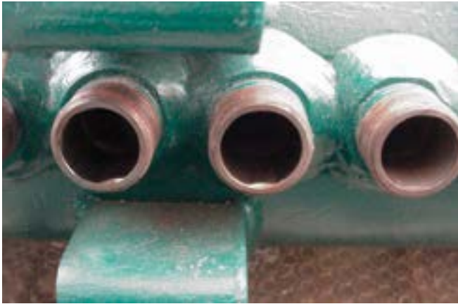
MiniSCALEMASTER nipples at very narrow pitches with overlapping weld seams
